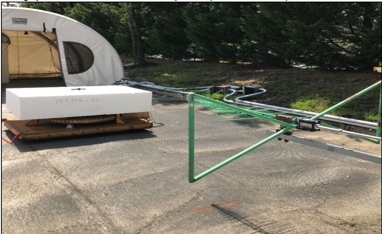
Photograph 4: Radiated Emissions Test Setup – Rear (30 MHz – 1000 MHz)
