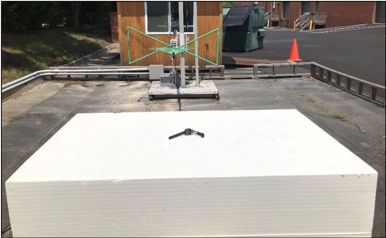
Photograph 4: Radiated Emissions Test Setup – Rear (30 MHz – 1000 MHz)
