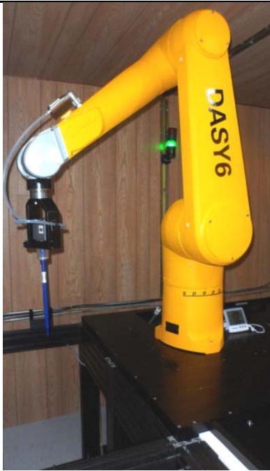
DASY 6 SAR System with SAM Phantom
